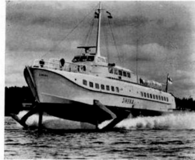
OUR COVER PICTURE SHOWS SIRENA, one of the Supramar PT 50 hydrofoil boats plying between Stockholm and the Finnish Aland Islands. Equipped with two Daimler-Benz diesel engines of 1,350 h.p. each, the Sirena seats 120 passengers.
